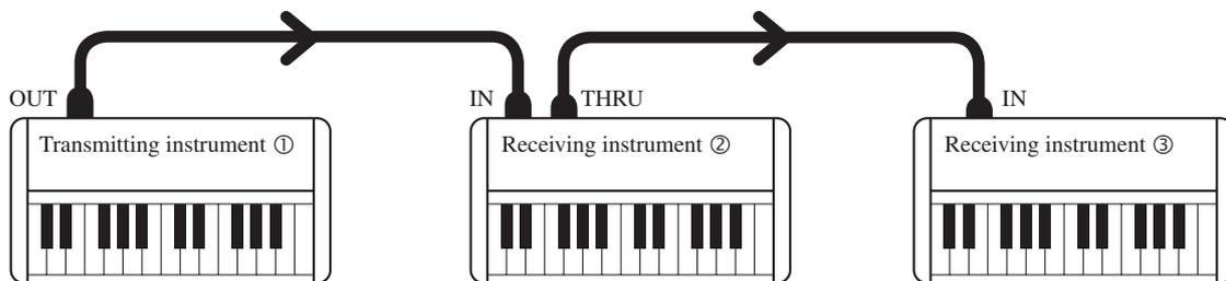
The information arrives at the receiving instruments ② and ③. Receiving instruments ② and ③ will respond to MIDI data that is sent if their receive channel is the same the transmit channel of transmitting instrument ①. If the channels do not match, then the receiving instruments ② and ③ will not respond to any data that is sent.
